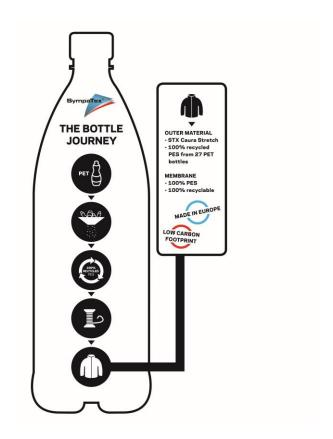
The outer materials that are made of recycled yarns represent up to 90% of a final Sympatex laminate product. They are a 100% recyclable product due to the 100% recyclable PES membrane. The performance of recycled and non-recycled PES materials is comparable at a high level.
